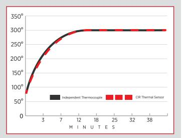
CPAC's CIR™ Thermal Sensor has been validated through thermocouple comparisons to be within 0.5 degrees F as measured on stainless steel instruments during sterilization cycle trials.
