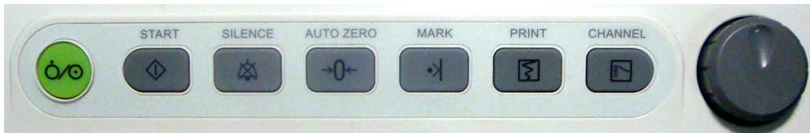
Figure 2-6 Keys and Control Knob
