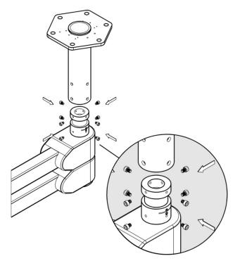
Figure 5: Installing the Central Axis on a 110mm Down Tube
