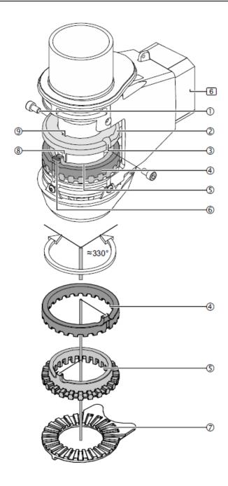
The swivel range of the Extension Arm [6] is defined by the position of the 3 end stops (2) / (4) / (5) engaged lightly with each other.
