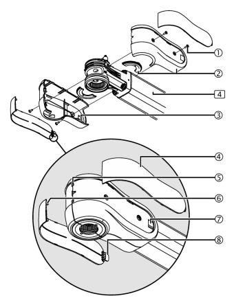
Figure 42: Dismantling the decorative caps and socket covers from the Extension Arm
