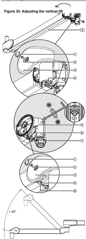
The vertical lift can be adjusted from approximately 0° to + 45° in the upwards direction.
