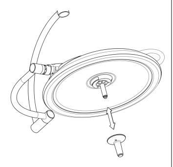
Figure 41: Handle Sterilization
