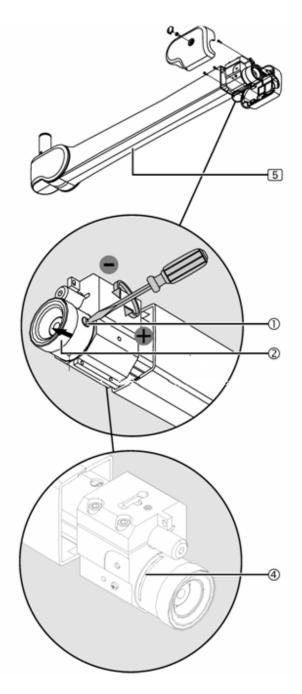
Figure 36: Adjusting the optional brake
