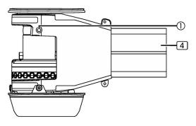
Figure 24: Adjusting the Extension Arm brakes
