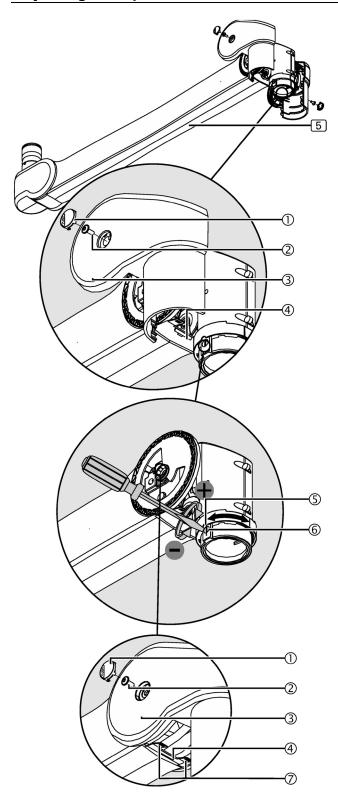
Figure 34: Adjusting the optional brake
