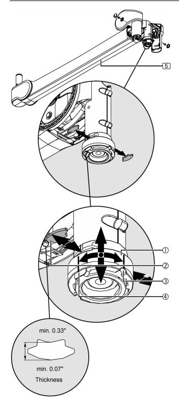
Figure 47: Checking the securing segment
