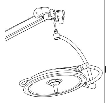
Figure 12: Mounting the Light Head
