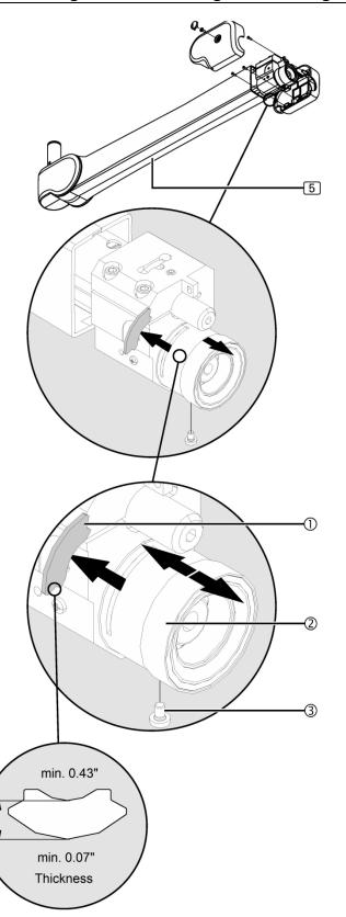
Figure 49: Checking the securing segment
