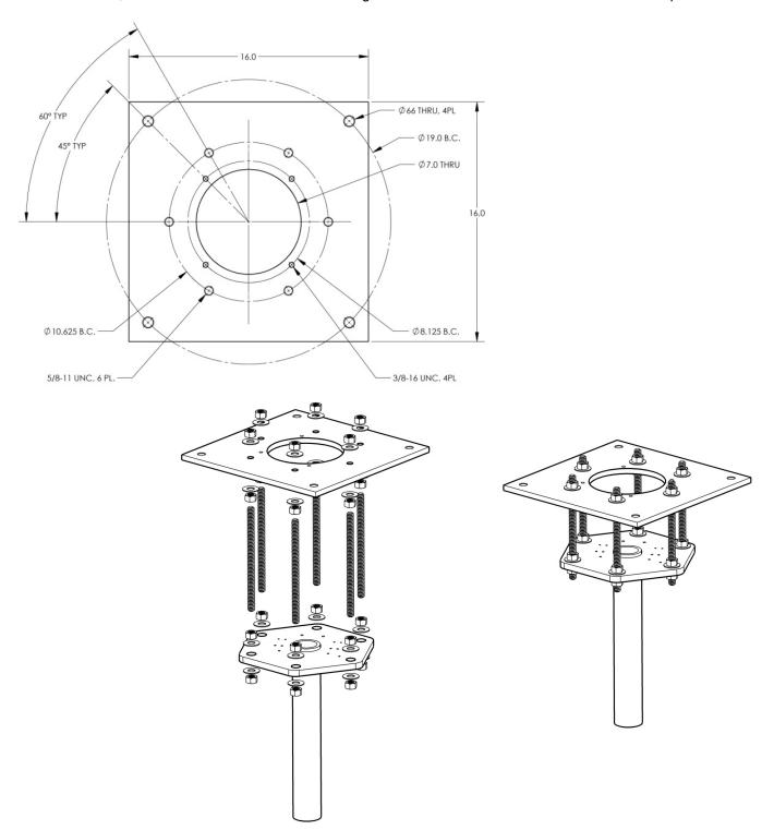
Figure 1: Ceiling Plate preparation with an Interface Plate
