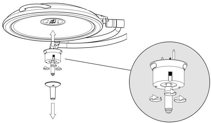
Figure 38: Attaching the Sterilizable Handle
