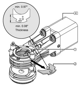
Figure 43: Dismantling the securing segment
