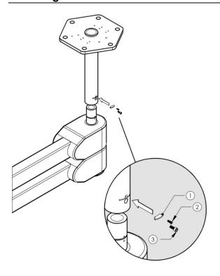
Figure 4: Installing the Central Axis on a 65mm Down Tube
