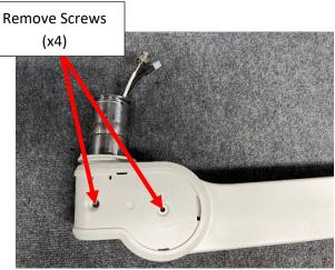
Figure 15: Preparing LCH Spring Arm with Camera - Screw Removal
