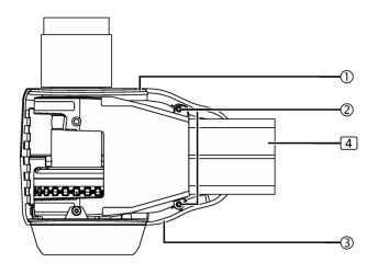
Figure 26: Mounting the left-hand cover panel to the Extension Arm
