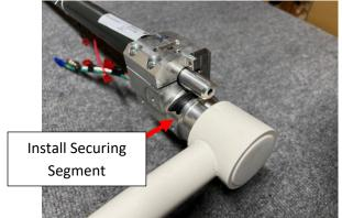
Figure 20: LCH Light Head with Camera - Install Securing Segment
