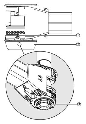
Figure 51: Checking the securing ring on the bottom Extension Arm towards the spindle
