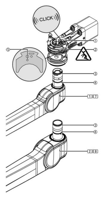
Figure 8: Mounting the L17 and LCH Spring Arms
