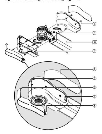
Figure 45: Mounting the socket covers and decorative caps to the Extension Arm
