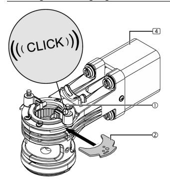
Figure 44: Mounting the securing segment
