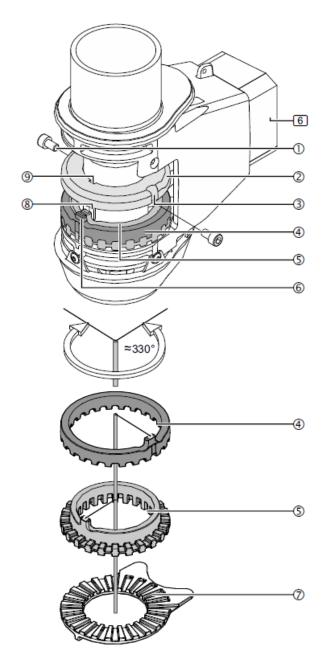
Figure 30: Adjusting the Comfort Stop end stop on the Extension Arm
