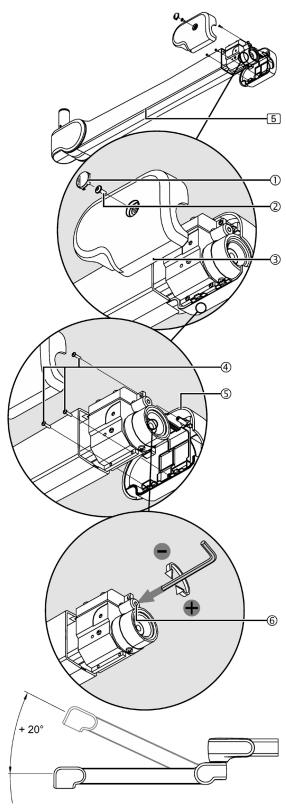
Figure 35: Adjusting the vertical lift
