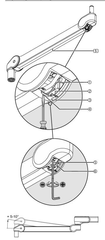
Figure 32: Adjusting the spring tension
