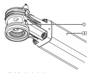
Figure 28: Adjusting the brakes
