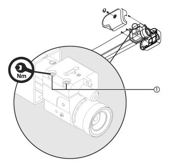
Figure 50: Checking the fixing screws on the Spring Arm I CH17
