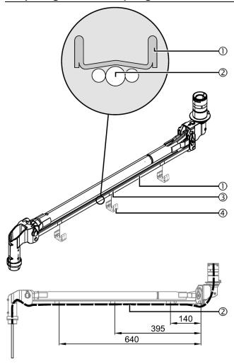
Figure 10: Mounting external cables
