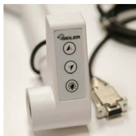
Remote switch and signal cable
