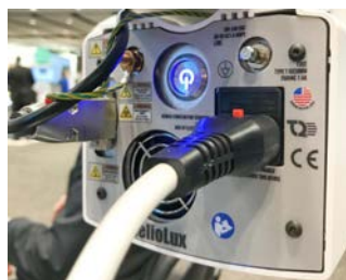
Remote cable connection to illuminator
