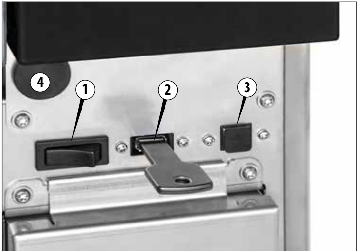
Fig. 13 - 1) ON-OFF switch. - 2) USB pendrive socket for PC connection and to use the «Win Tuttnauer Service tool wash» program. - 3) USB pendrive socket for inserting or extracting the pre-filled programs. - 4) Rubber cap to close access to the emergency release.
